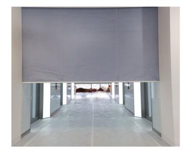
containment systems prevent spreading of smoke from one zone to another. Curtain comprises of flexible heat resistant fabric with fire integrity up to 240mins.\*. The tube contains a DC electric motor which holds the curtain retracted at ceiling level at all times and deploys upon the receipt of fire alarm signal. The bottom bar ensures safe and controlled descent of the curtain with gravity fail safe.
